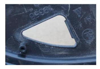
To fit perfectly our O3-MRLGT lights, you must cut it easily with knive:
